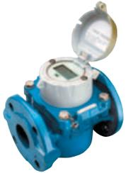
Range: 40/50/80/100/150mm. Innovative measuring technology ensures wide measuring range (better than most combination meters). Electronic register with integral pulse output provides versatile outputs and informative display. Interchangeable internal mechanism. H4000 body can be retro-fitted with H5000 internal mechanism 40-100mm only. Suitable for forward and reverse flow measuring. Pressure tapping. Max working pressure: 1 600 kPa. Battery life up to 15 years.
