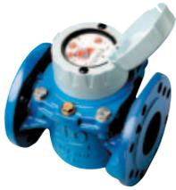
Range: 40/50/80/100/150/200/250/300mm. Interchangeable internal mechanism. Suitable for forward and reverse flow measuring. Versatile bi-directional inductive pulse output with external PR7. Pressure tapping. Max working pressure: 1 600 kPa.
