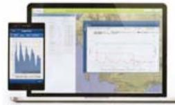
Flow and pressure logging. Web based interface. Suitable for any pulse output water meter. Data import and export. Alarms. Automated reporting. Interactive geographic maps.
