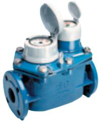
Consisting of an H4000 Woltmann helical vane inferential type water meter and an integral V220 class C bypass meter. Range in mm: 50/80/100. Max working pressure 1 600 kPa.
